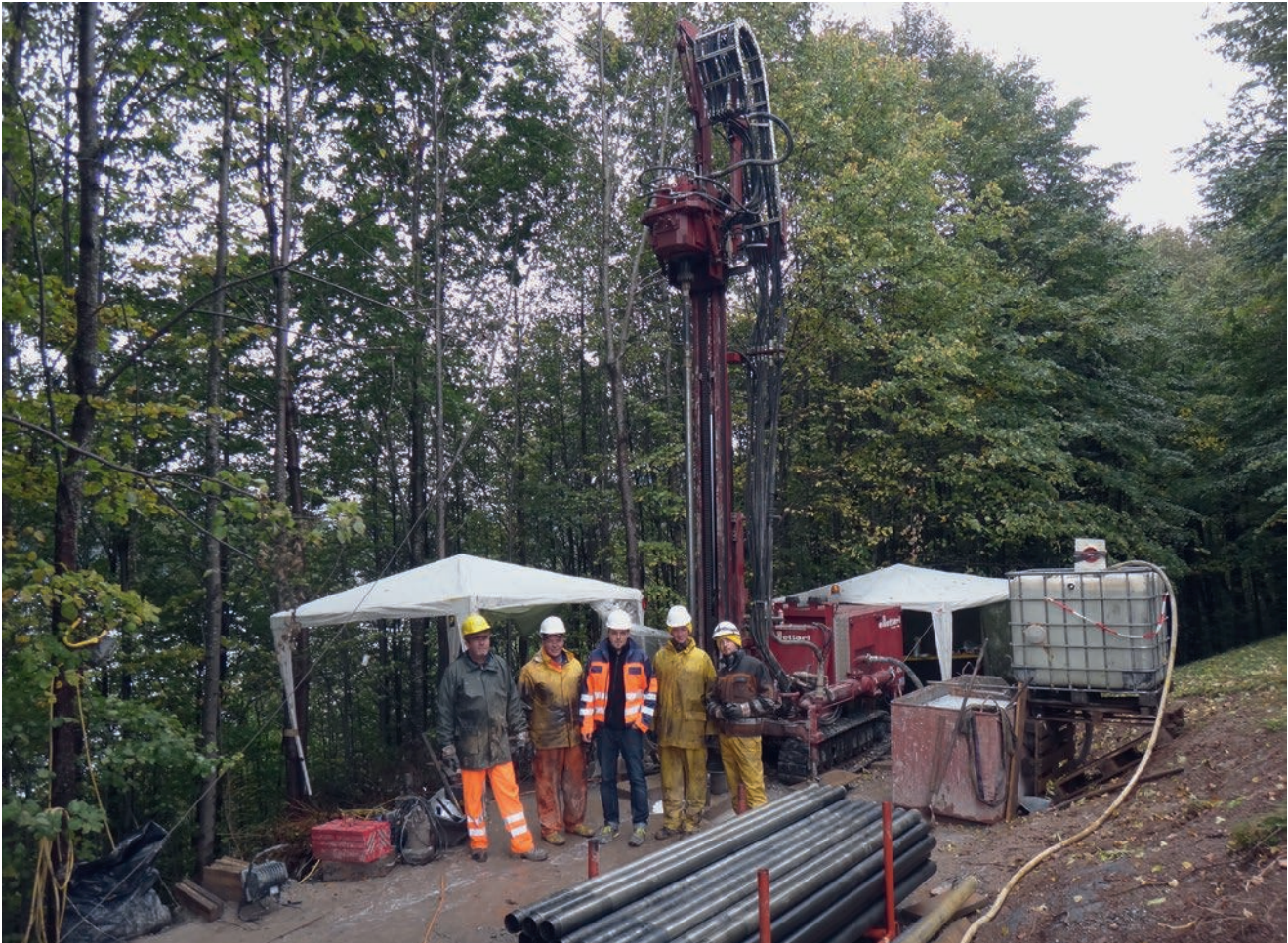
Drilling site for the 300 m-deep exploration hole in difficult terrain
